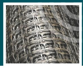
Interlock Geogrids are manufactured from highly orientated (punched and stretched) monolithic polypropylene sheets with integral nodes, specifically for the reinforcement and stabilisation of unbound granular soils. The junctions and rib geometry facilitate mechanical interlock with the granular soil layers.
